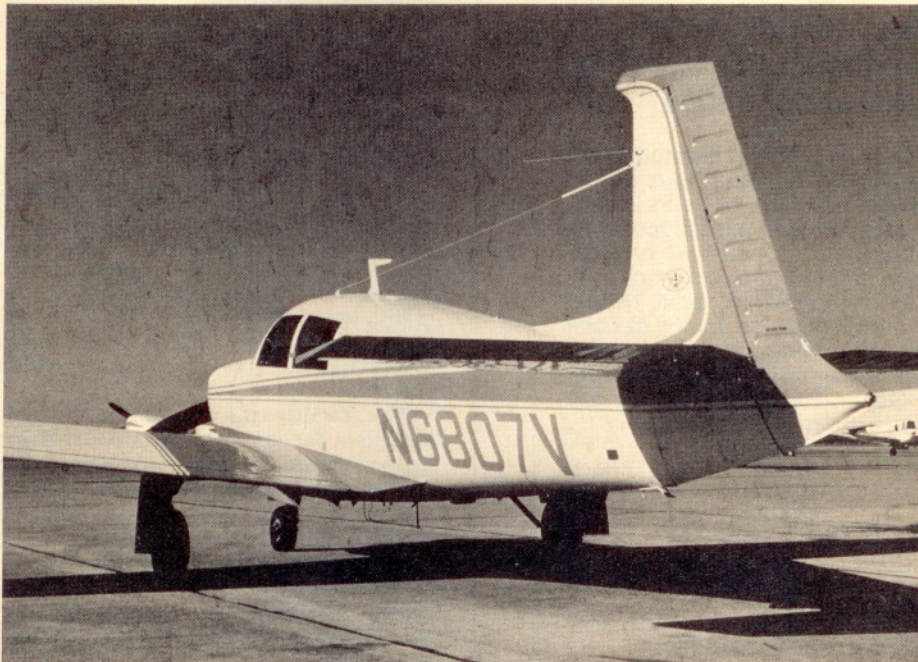
The last Mooney Chaparral built prior to the plant's shutdown in 1971 displays the "stinger" and counterbalancing "beak" added by Butler Aviation. These features will not be retained on the new models, which will get a new paint scheme and a redesigned instrument panel.
